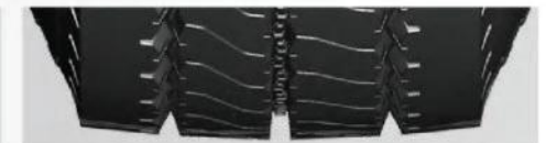
Optimized tire grounding marks design prevents irregular wear
