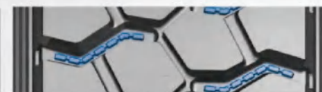
Anti-clamping stone design
