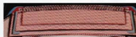
High strength stiffness steel belt structure
